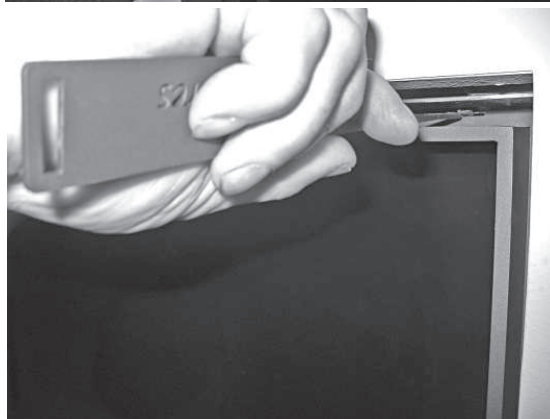
- With the hook, pull the thin, metal spring strips on the top left and right from the studs on the frame.
