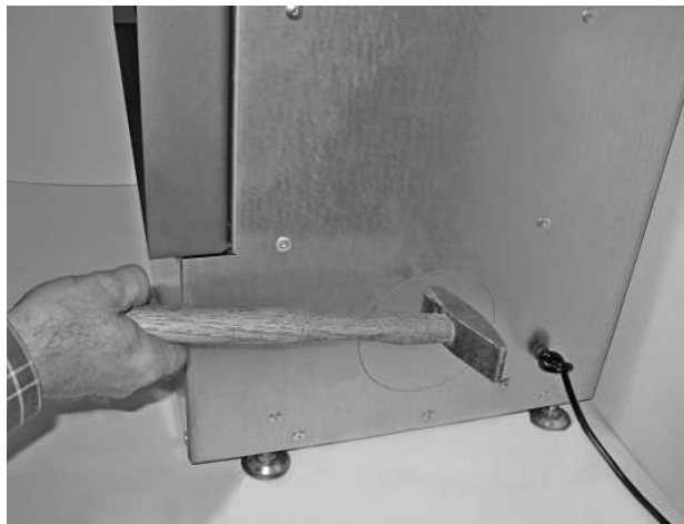
Breaking out an opening on the side
